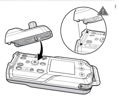
i Alternatively the pump adapter can be used with an on-demand valve.
