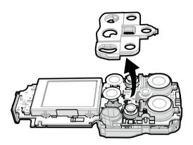
b. Place the special tool on the trough. Using the accompanying special tool (1), carefully lift out the desired EC sensor (2). Do not bend the sensor pins.
