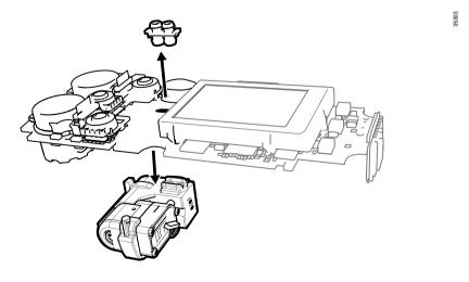
9. Pull pump out of pump block.
