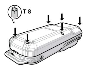
3. Carefully pry apart the front and rear housing cradles (e.g. with a coin).
