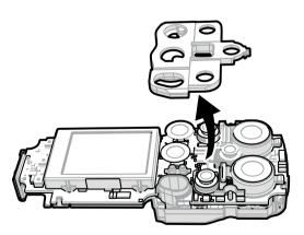
4. Insert a new sensor sealing plate of the same type (press it into the double tube area (only with pump)).
